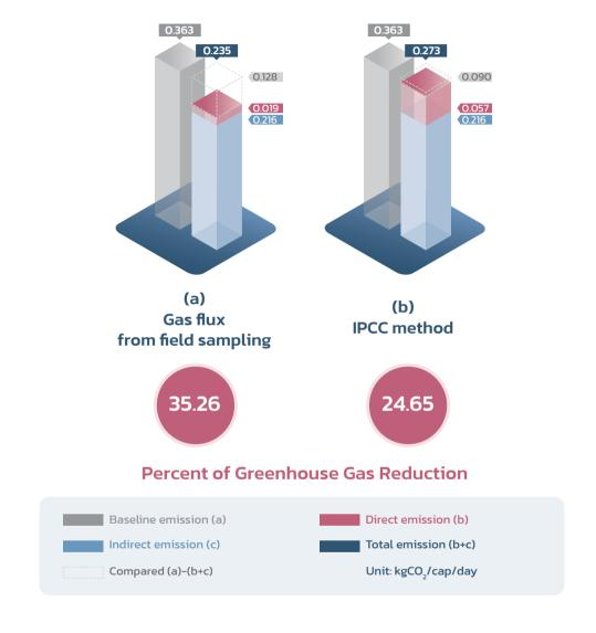
However, when the direct greenhouse gas emissions from the aeration septic tank system from field measurement and calculation are combined with the indirect emissions from electricity consumption and compared with the baseline, the emission reduction is 35.26% and 24.65%, respectively.
