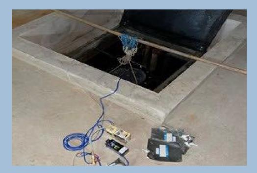
Figure 3.6 Gas sampling method from septic tank aeration system
