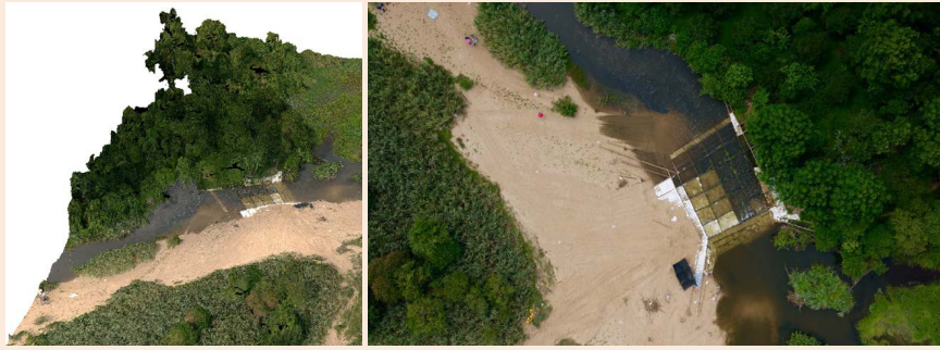
Figure 1: Example of the SfM data processing workflow from the Tha Di living weir, shown as a textured 3D model on the left and aerial picture of Living Weir construction site on the right
